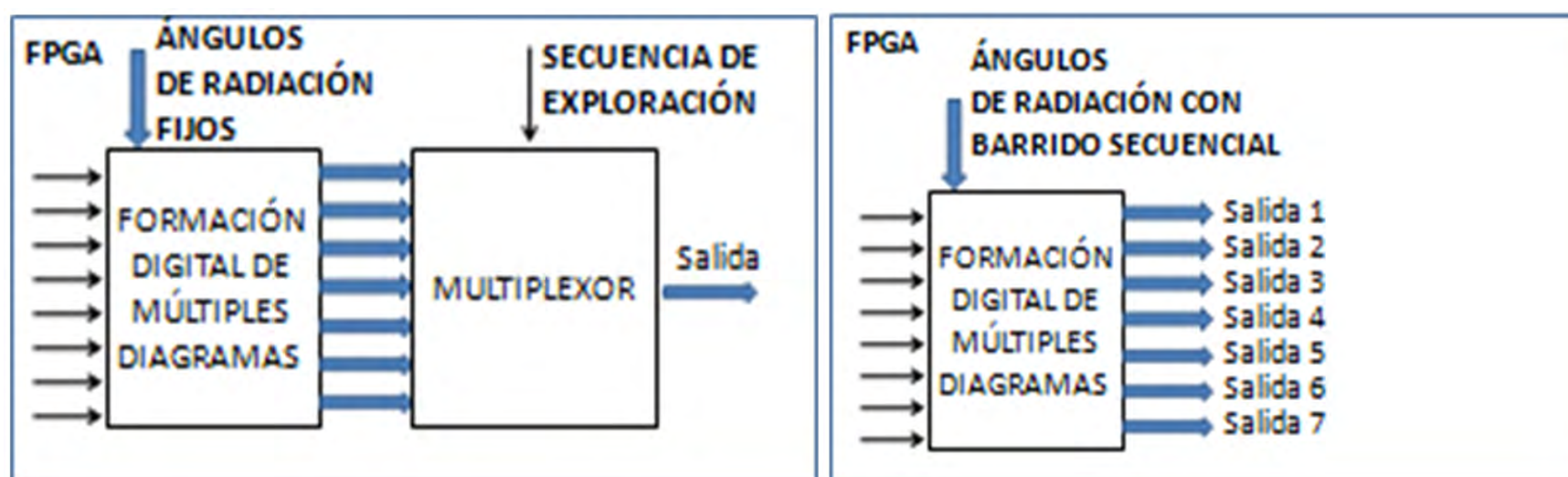
Figure 3. Beam switching system.
