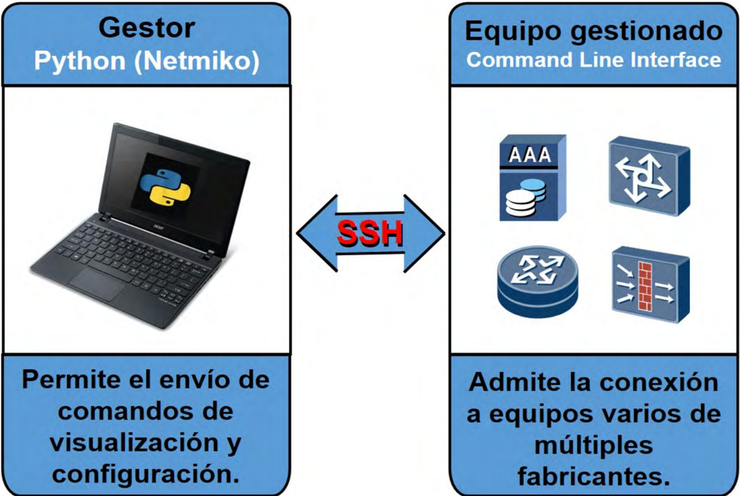
Figure 2. Network automation using Netmiko
