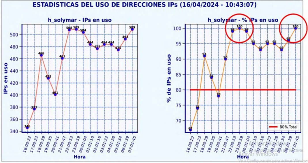
Figure 6. Under-dimensioned IP Pool Behavior
