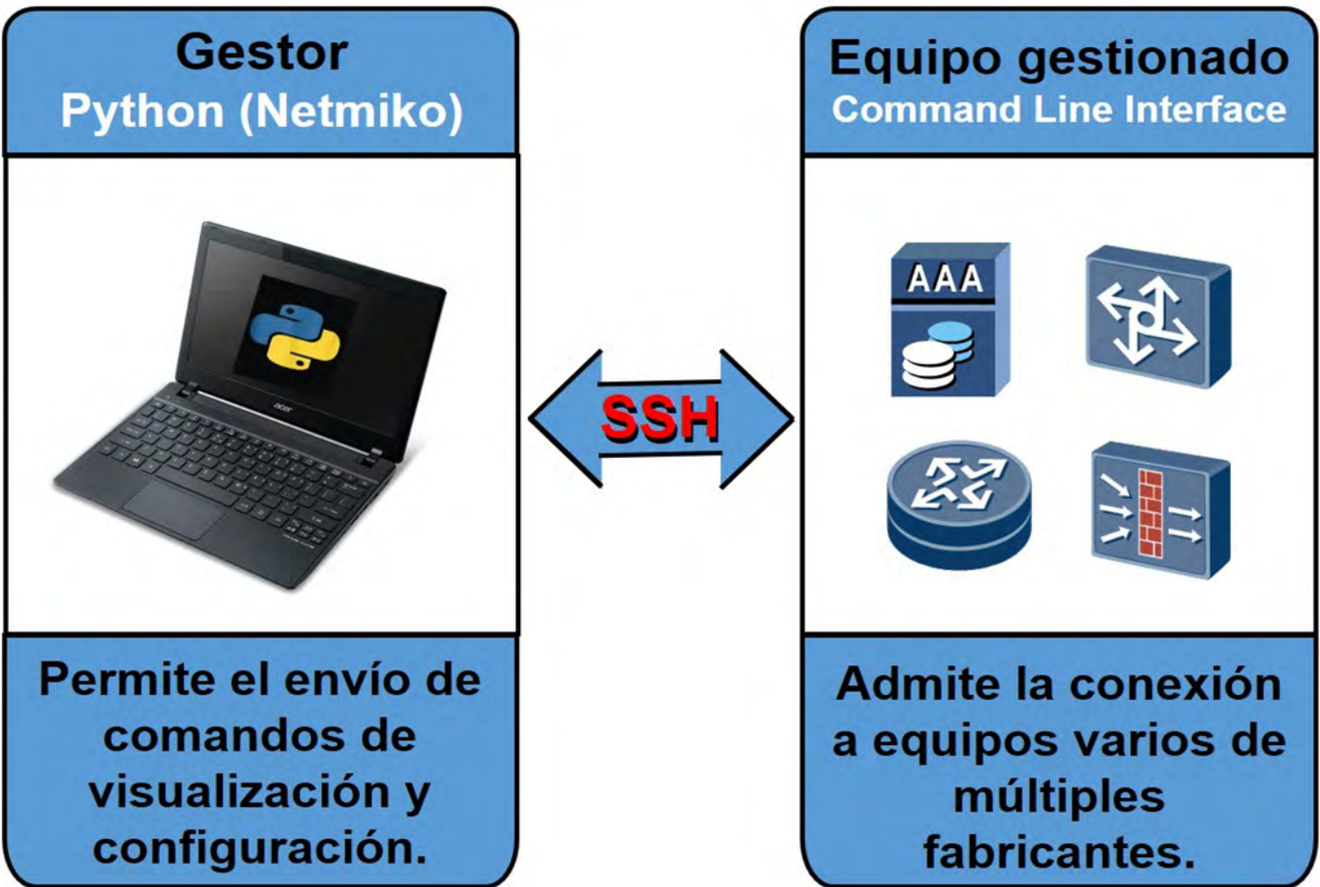
Figure 2. Network automation using Netmiko
