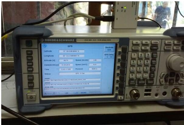
Figura 7. Receptor satelital GPS.
